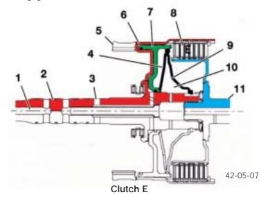
Free wheel gearshifts (using overrunning clutches) are not used in this transmission. In the GA6HP26Z gearbox, all gearshifts from 1st to 6th gear and from 6th to 1st gear are executed as overlap shifts. The overlap gearshift system saves weight and space. The electrohydraulic gearshift is executed by valves in the valve body that are controlled by pressure regulators. The speed, pressure and torque curves are shown in the following diagrams.
